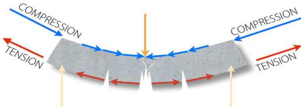
Figure 2: A simply supported concrete beam reacting to a point load.
