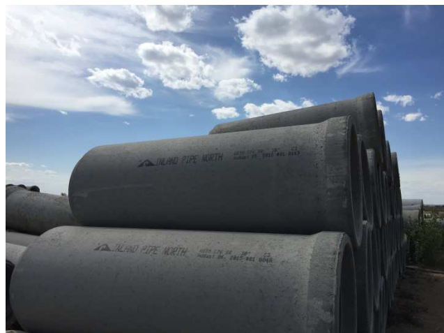
Figure 1: All precast concrete products that meet the strict PPP requirements are stamped with the program logo, a black triangle with a "P" inside.
